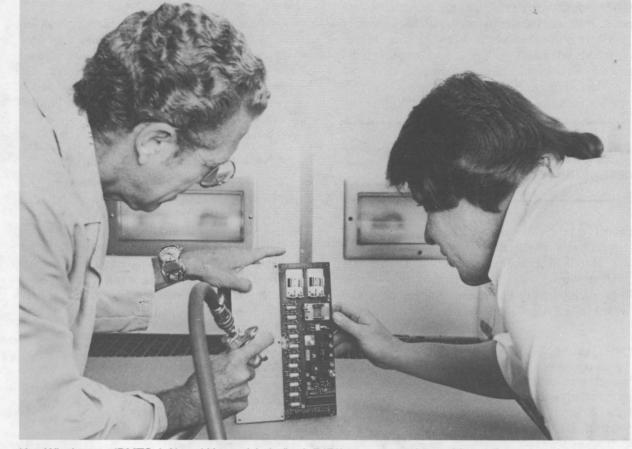
Ken Wischmann (DMTS, left) and Howard Arris (both 7472) spray a tough epoxide coating on an electronics assembly. The coating, developed by Ken and Howard, cures within a minute in a special ultraviolet apparatus designed and built by John Sarkis (2852). The non-proprietary coating formula is one of Sandia's all-time tech transfer "best-sellers."
